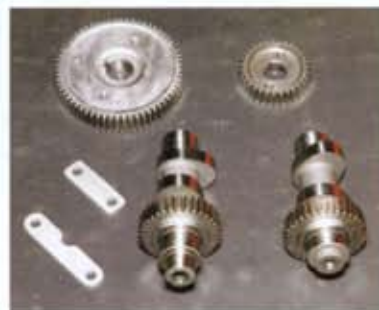
The S & S camshafts feature their unique gear drive system. The kit includes block-off plates that replace the two hydraulic drive chain tensioners.
