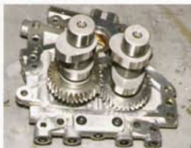
The S&S gear drive camshafts do away with the stock intermediate drive chain and hydraulic tensioner. Because the gear drive rotates the cams in opposite directions, the system also allows for higher lift without the lobes running into each other.
