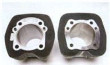
The Revolution Performance cylinder (right) is cast from aerospace-grade aluminum. It does not use a steel liner like the stock cylinder on the left. The internal cylinder wall is given a nickel-silicone-carbide coating. This makes the cylinder bore harder than steel, with excellent wear properties.
