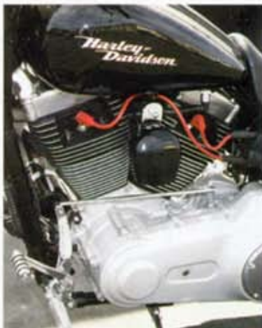
To give the motor a sharp contrast, County Line used black cylinders and heads instead of the natural aluminum finish that came on the Super Glide. This went well with the other blacked-out parts on the bike.
