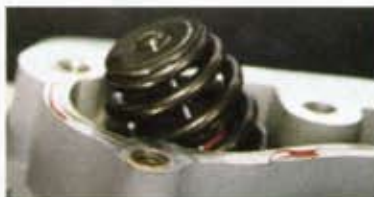
The interference is caused because the stock cylinder heads use "beehive" shaped valve springs with small diameter retainers.
