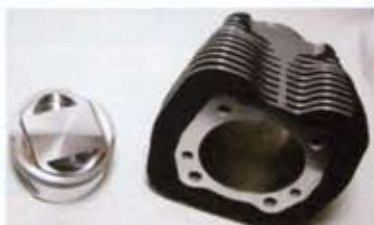
Our big-bore kit included a set of forged pistons made by CP Pistons. The pistons have a raised crown that gives the motor 10.2:1 compression when used with a stock size Twin Cam combustion chamber. They also offer a big-bore kit for Harley's 96-inch 2007-up motors that gives them 107-inches of displacement.
